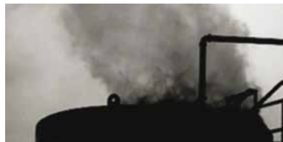
To the naked eye, no emissions from an oil storage tank are visible (left), but with the aid of an infrared camera, escaping CH 4 is evident (right).
