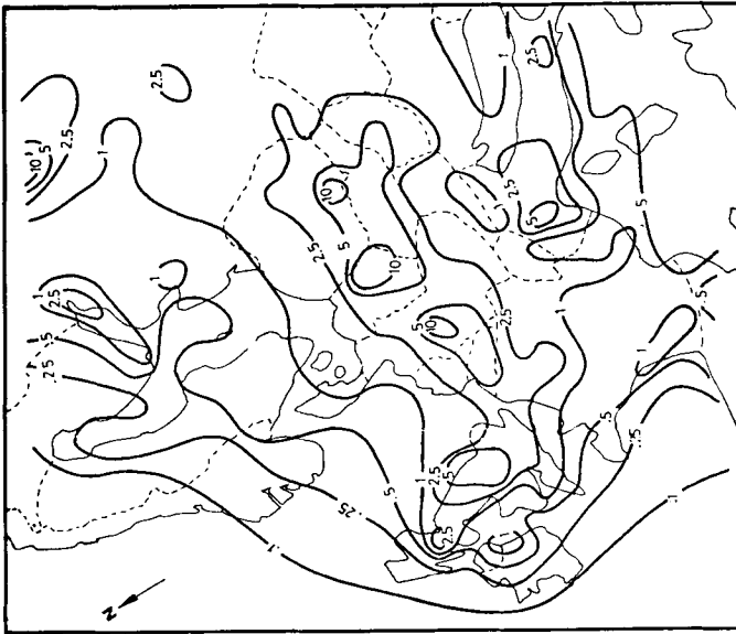
Figure 4 (a). Calculated sulphur dry deposition patterns in western Europe for 1974 (OECD 1977). Unit: \text{g S m}^{-2} .
