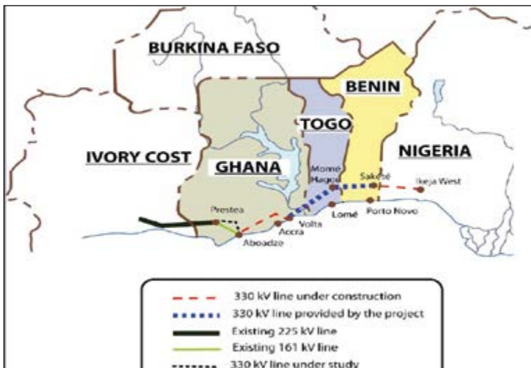
Figure 18. Coastal backbone interconnection
