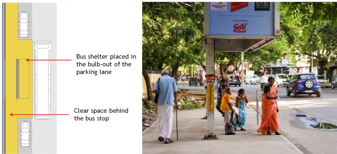
Figure 9: Bus stops should be placed adjacent to buses' linear line of travel and should allow for continuous footpath and cycle tracks.
