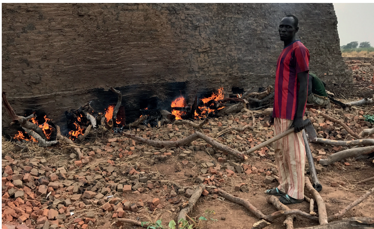
Use of Mahogany wood for bricks making in Aweil. Photo Credit: Arshad Khan, UN Environment.
