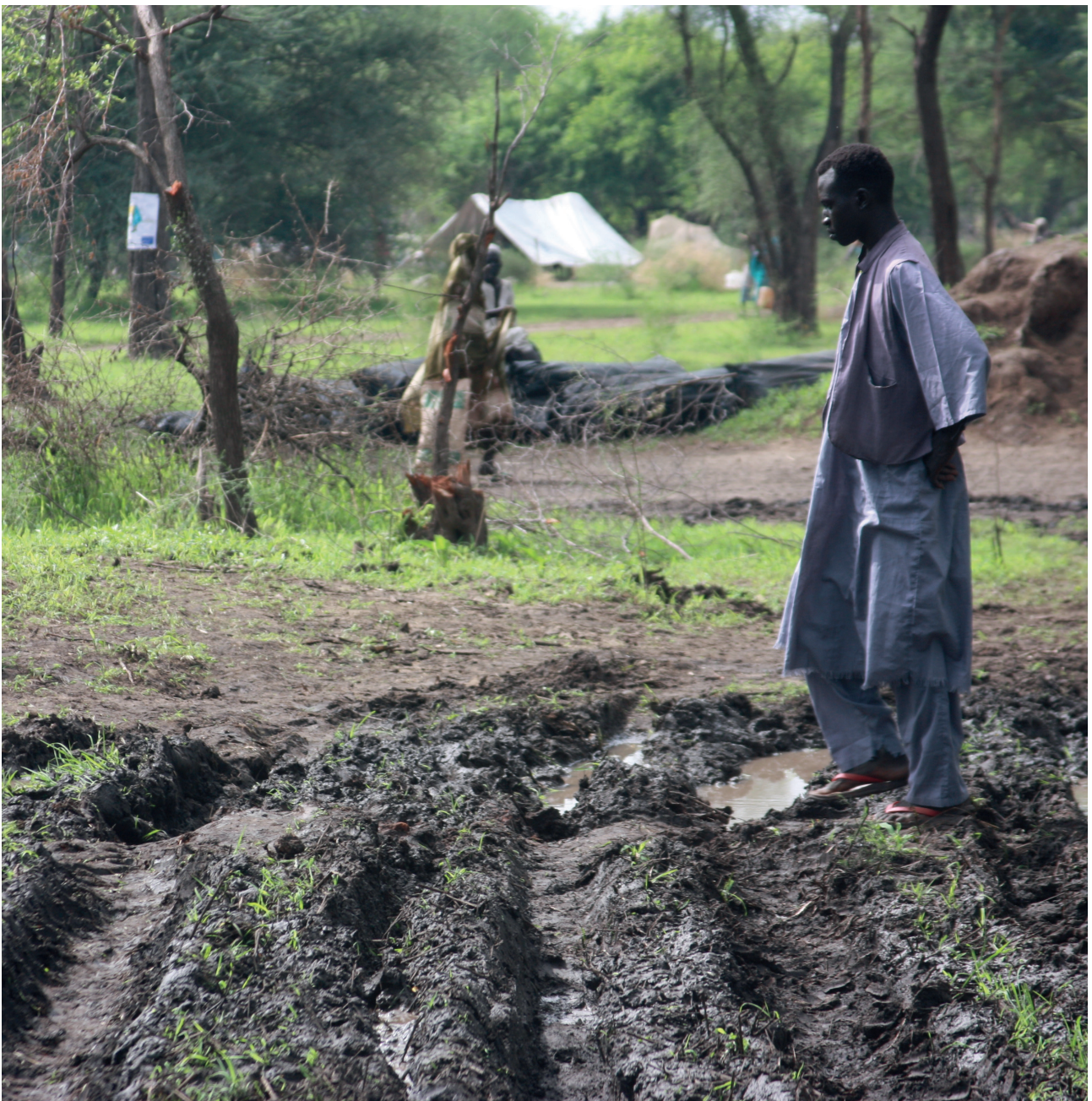
Black cotton soil with the rain makes roads and airstrips unusable. Photo credit: Amy the Nurse/Flickr.com/CC BY-NC
