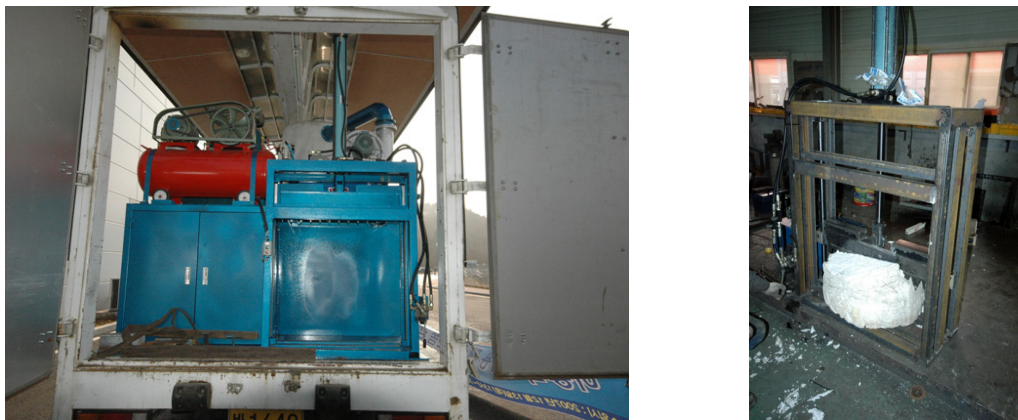
Fig 3. Hydraulic cutter for large buoy. (a)Buoy cutter loaded on the truck(left) (b)Large buoy cutting test(right)
