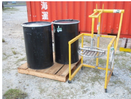
Fig 2. Drum can containing solvent and manual volume reduction equipment for drum can.
