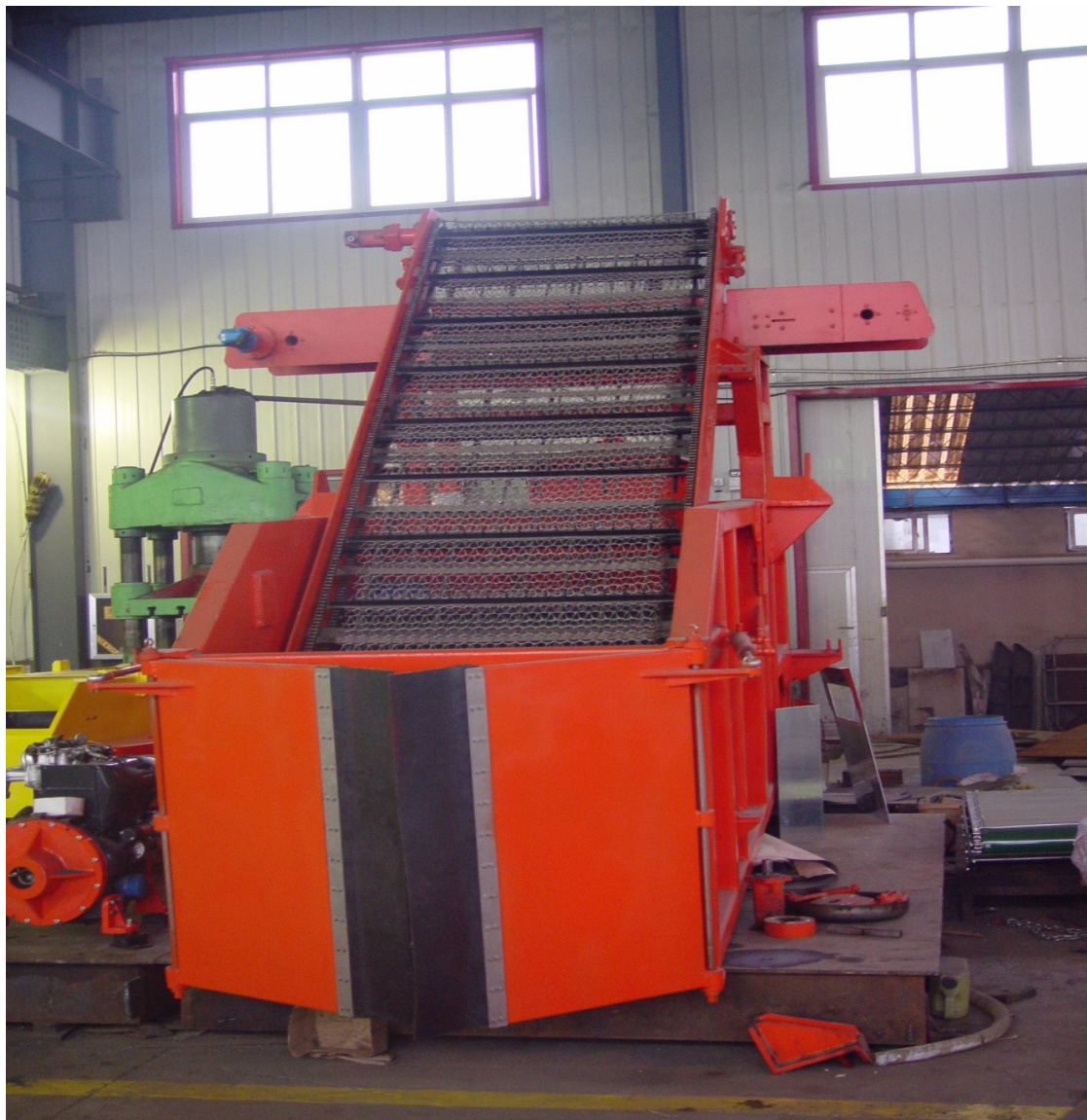
Fig 2. Upward rolling system of the SGRE.
