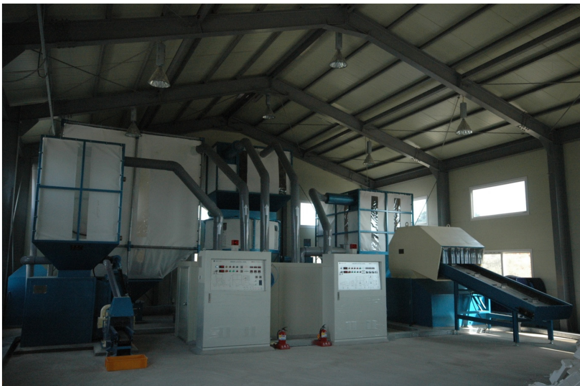
Fig 2. Used polystyrene buoy thermal volume reduction system.
