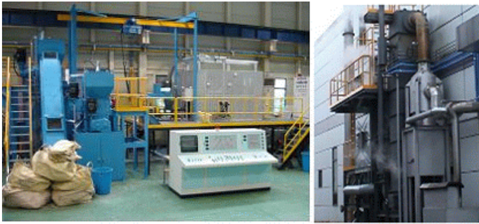
Fig 2. Pilot plant for the FRP vessel melting treatment and the anti-air pollution facility.
