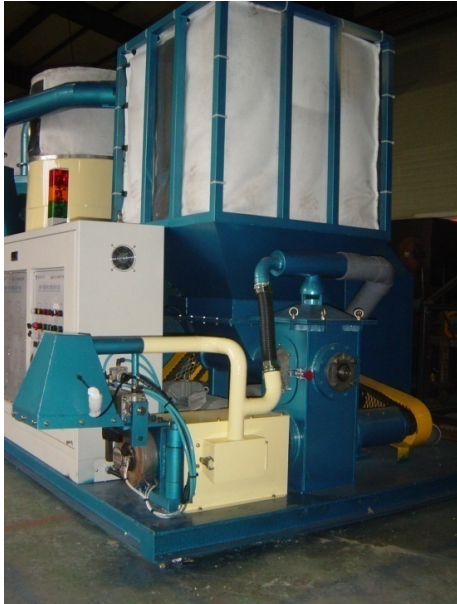
Fig 7. Injection molder (30 kg/hour).
