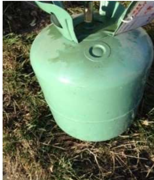
Unlabelled refrigerant cylinders containing R22
