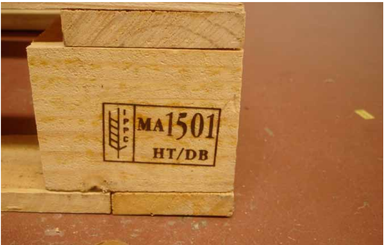
A wooden pallet from Morocco with the required IPPC stamp showing it was heat treated (HT)
