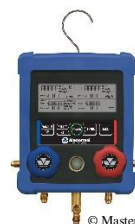
Electronic manifold gauge set that can be used with flammable refrigerants, ammonia and high pressure refrigerants (up to 50 bar)
