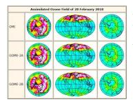
TEMIS -- Near-real time global ozone field. The in near-real time delivered total ozone columns, derived from satellite observations, are input to a data assimilation program which provides global ozone fields for today and a forecast for the coming days.
