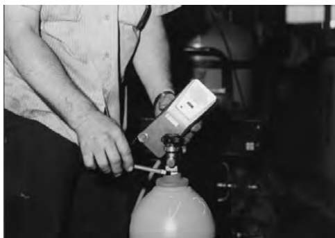
Photo 7-3. Example of a leak detector.
