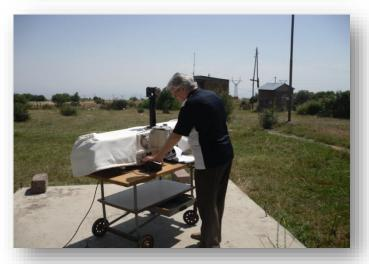
Representatives of the Hydrometeorology Service the Dobson presented device, spectrophotometer on-site measurements were carried out by the Ozone-Measuring Station employee. The Head of the Helio-pharmacology and Atmospheric Studies Division of the Ministry of Emergency Situations, Anna Tsarukyan presented the data processing techniques. Other equipment and their significance were also presented to the participants.
