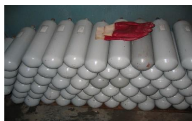
Mercury flasks at the mercury recovery plant Kubantsvetmet in Krasnodar (Photo credit COWI)
