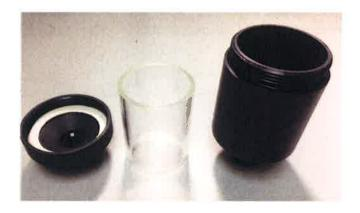
The adsorbents may vary depending on the analytes suitable to be collected: polyurethane foams (PUF), polymeric resins (such as amberlites) or activated carbon. Adsorbents placed into the adsorbent module will capture the gas fraction of the air sample. In the process described in this procedure, the combination of 2 PUF (with different size) and polymeric resin XAD-2, accommodated in a glass holder, is used.
