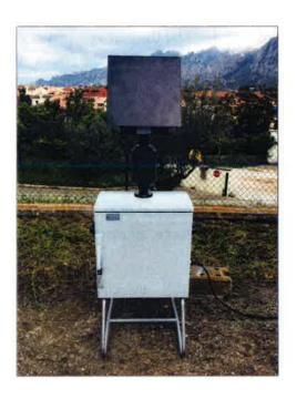
This configuration makes reference to the 'MCV type' sampler, which is the one used by the CSIC, and it is possible to observe slight variations in comparison to other sampling devices, although all of them are based on the same principle, such as those used, for example, in POPs Monitoring Project in East Asian Countries, MONET, GAPS, GAPS-GRULAC, GMP-UNEP and EMEP Program.
