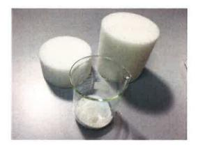
First step consists in placing the smaller PUF inside the glass holder, followed by 10 g of the polymeric resin (XAD-2) and finally the larger PUF to cover and sealing the system.
