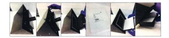
NOTE: In order to avoid contamination episodes, analyst must wear protection gloves during the placement of the filter. A couple of clean tweezers can also be used to help to properly place the filter on the support surface. It is important to avoid dusty and/or dirty working areas.
