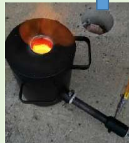
Small furnace melting at 1,200 C°
