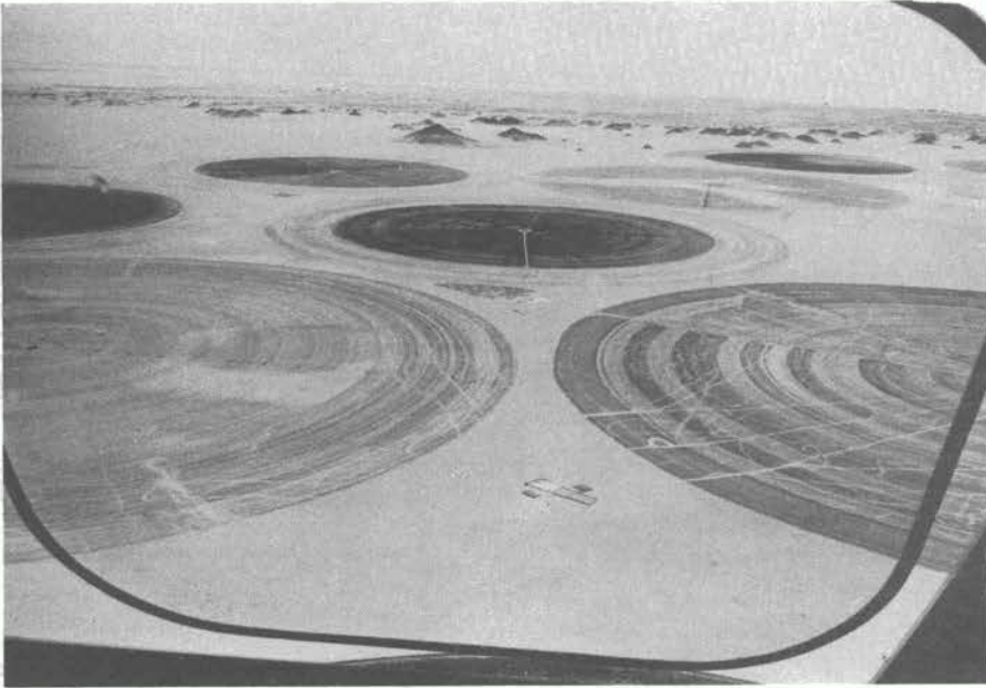
Figure 11.1. Pump irrigation at Kufra oasis, Libya. Each circle is watered from a 560 m long pipe, supplied with 76 litres of water/second and moving one turn in 24 hours. Very high costs and limited fossil groundwater supplies are two difficulties connected with similar projects. Air photo, S. Leijonhufvud.
