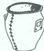
30 to 80 litre bin made from truck tires
