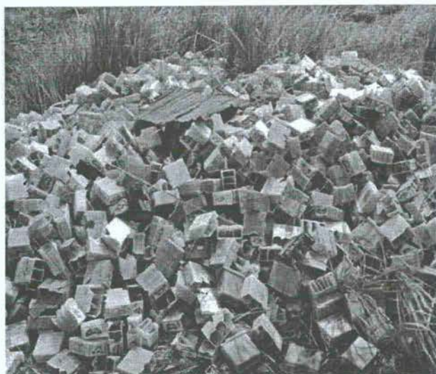
Picture 24: Battery cases after breaking
