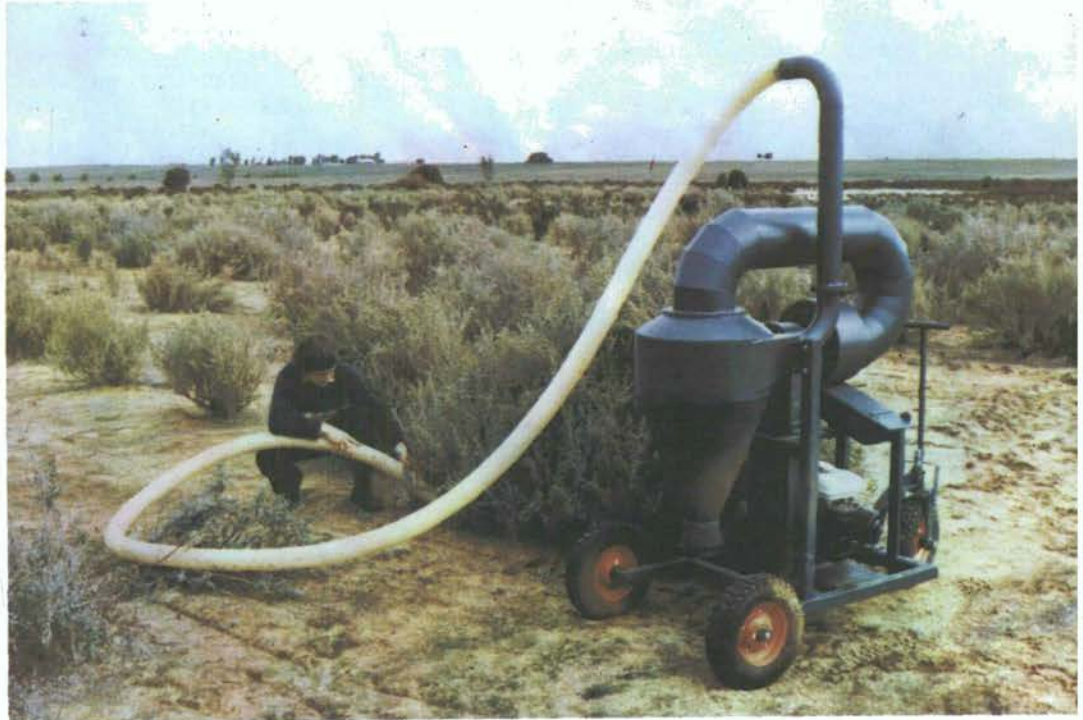
A low cost vacuum seed harvester used for collecting seeds for replanting. (Photo by John de Sallis)
