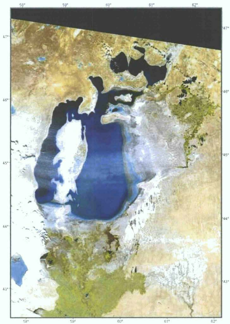
Fig. 32. Space image MODIS (spaceplatform TERRA), June 7, 2001, resolution 250 m, color composition of band 6, 2, 1, area of water mirror – 24,5 thousand km 2
