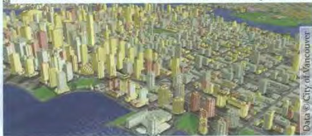
Color-coded city model showing how Autodesk® Infrastructure Modeler 2012 software can be used to theme existing GIS data.
