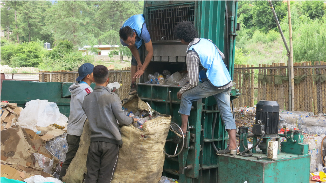
A group of men at Greener Way are compressing PET-bottles at the transfer station. Photo by Ieva Rucevska.
