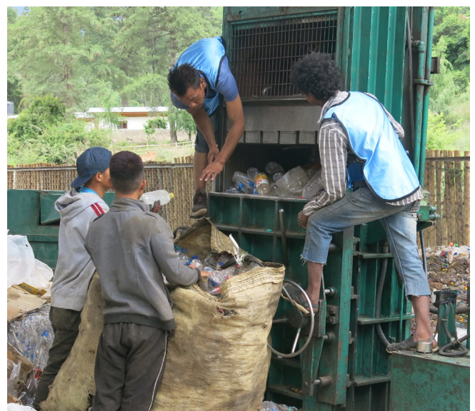
A group of men at Greener Way are compressing PET-bottles at the transfer station. Photo by Ieva Rucevska.
