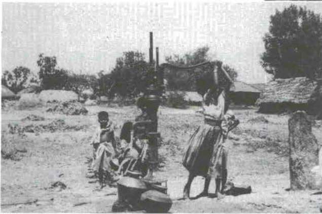
This girl operates pump comfortably, using almost entirely body weight. Resting position of handle, however is too high
