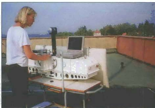
The Dobson ozone spectrophotometer D074 operated at the Solar and Ozone Observatory of the CHMI in Hradec Králové
