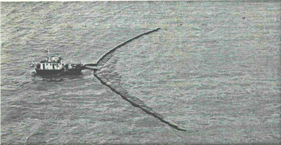
4. Separate tension boom under tow by two vessels with skimmer deployed from third vessel behind boom.
