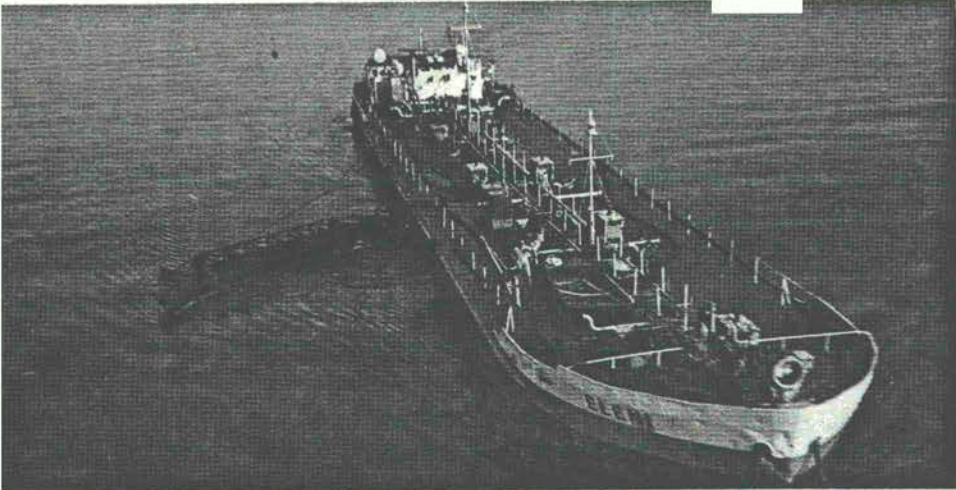
2. Single ship collection system employing a rigid boom deployed from small coastal tanker.
