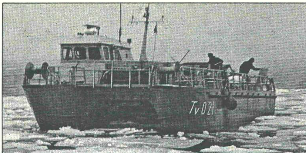
6. Catamaran-mounted disc skimmer operating in ice.
