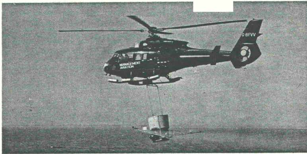
Figure 4. Helicopter bucket spray systems.
