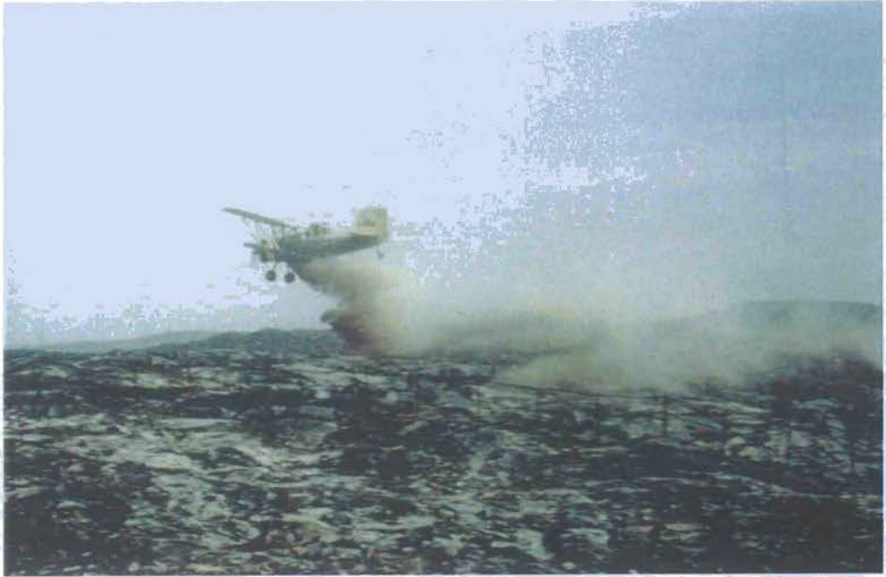
Picture 11 : Lime application to the site by air to increase the pH of the soil. The Site is a fume kill area.
