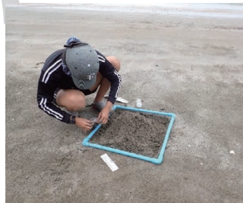
Figure 4: Placing a 0.5 m x 0.5 m quadrat on a beach for MP sample collection
