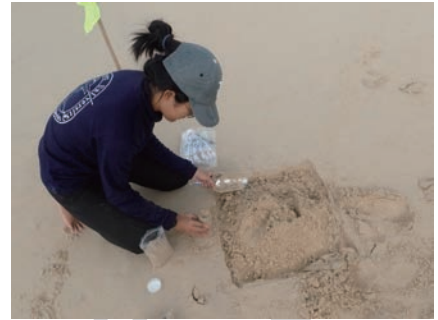
Figure 5: Taking sand samples from the top 2.5 cm of the quadrat area
