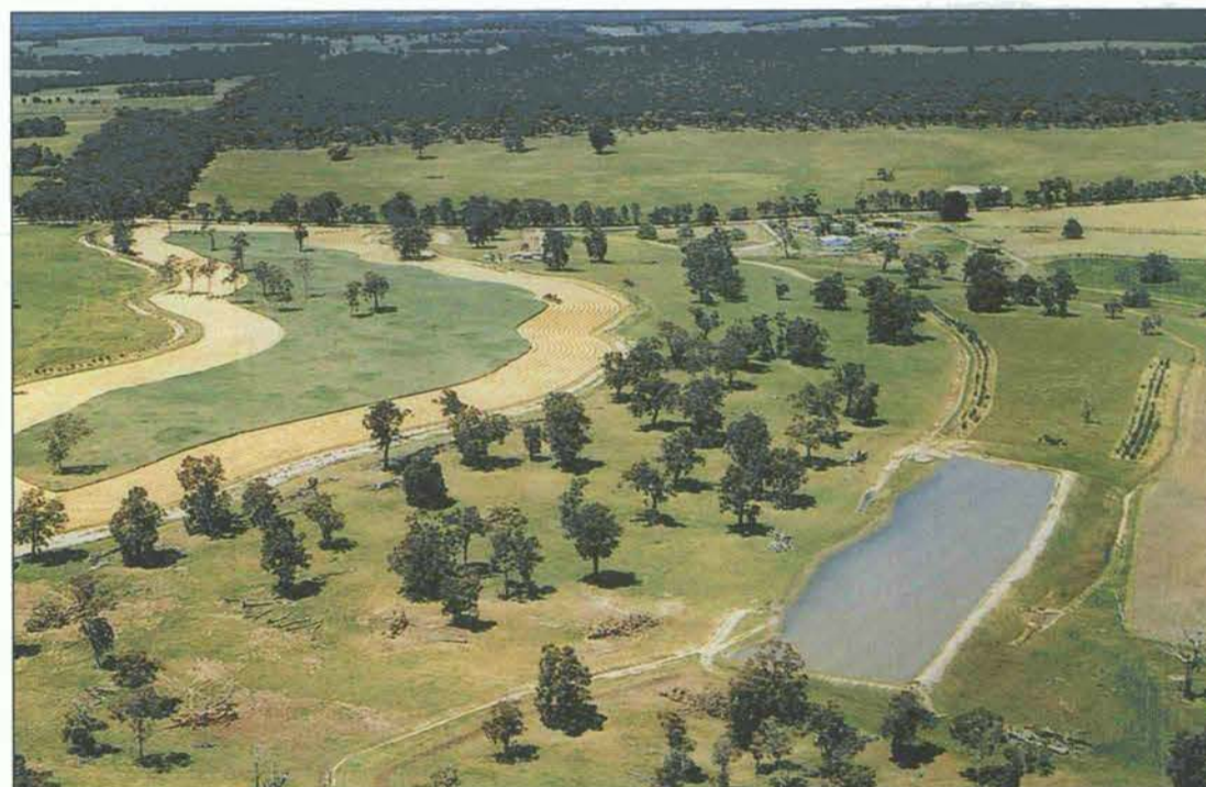
Figure 4.53 The interceptor drains lead into check dams that provide water for humans, livestock and irrigation
