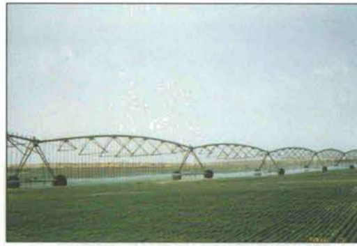
Figure 4.37 Centre-pivot boom irrigating the oilseed halophyte Salicornia with seawater (Jim Riley, Environmental Research Laboratory, University of Arizona)
