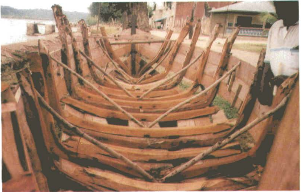
The ribs and keel of this large boat are made from mangrove timber
