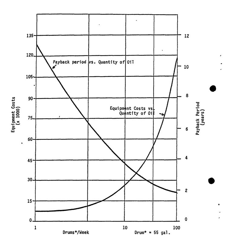
Figure 5.1 Equipment costs and payback period vs. drums of oils
