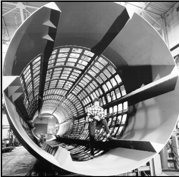
Figure VI-14. End view of a trommel screen
