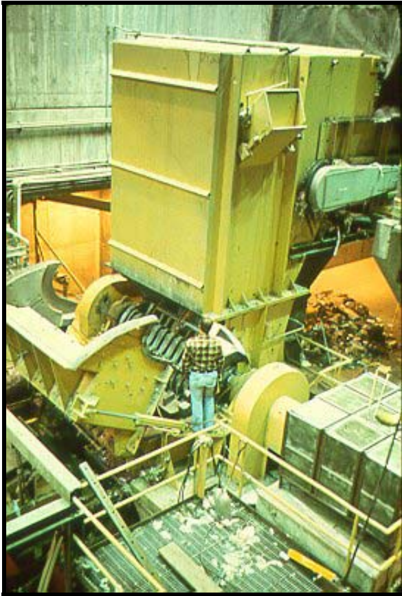
Figure VI-3. Commercial horizontal hammermill (centre, shown in opened position) with feed chute (top centre) and electric motor (lower right)
