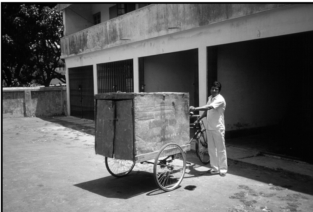
Figure IV-13. Modified pedal tricycle used for waste collection
