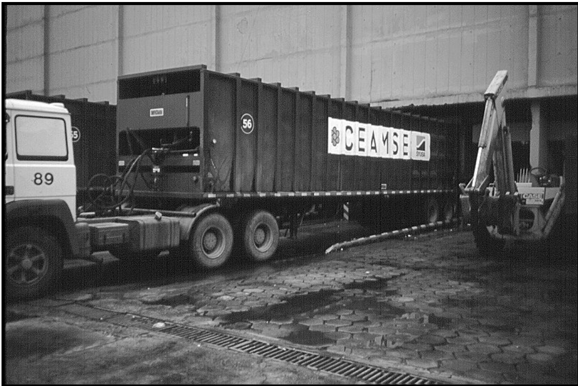
Figure IV-24. Transfer trailer being loaded by a compactor
