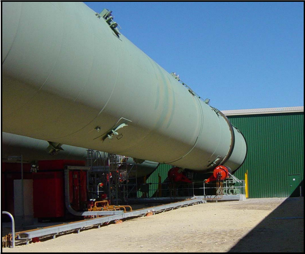
Figure VIII-8. Example of Eweson drum design (Western Australia)
