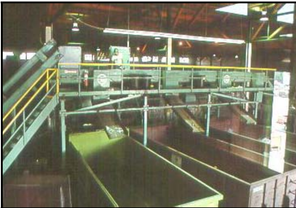
Figure VI-24. Example of a rigid container processing line at a source-separated processing facility
