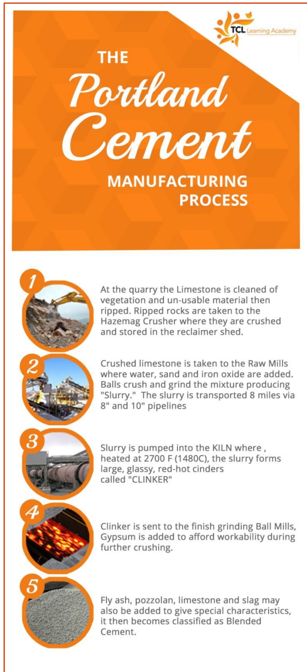
Figure 14: Outline of the cement manufacturing process (TCL, 2014)
