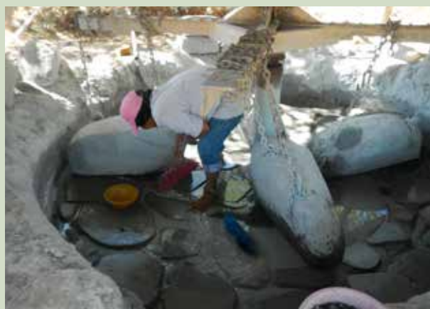
Whole ore amalgamation in a 'Rastra'. Mercury is added to all the material that is milled by the turning rocks.
