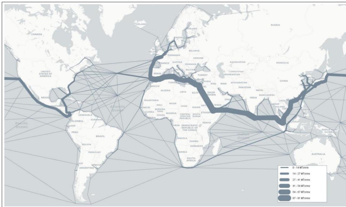
Figure 16: Visualisation of CO 2 Emissions projections across shipping routes in 2015; Source: ITF - Decarbonising Maritime Transport - Pathways to Zero-Carbon Shipping by 2035 — OECD/ITF 2018.
