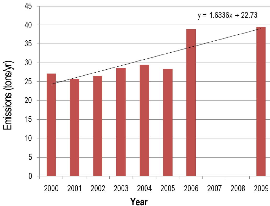
Figure 5: Historical estimated mercury emissions from coal-fired power stations in South Africa (after Masekoameng et al., 2010)
