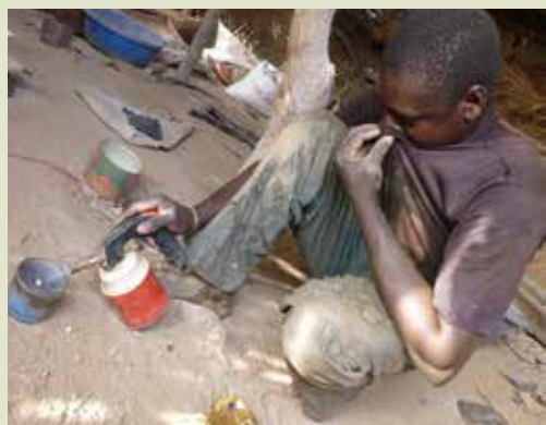
e. The amalgam is burned to evaporate the mercury
