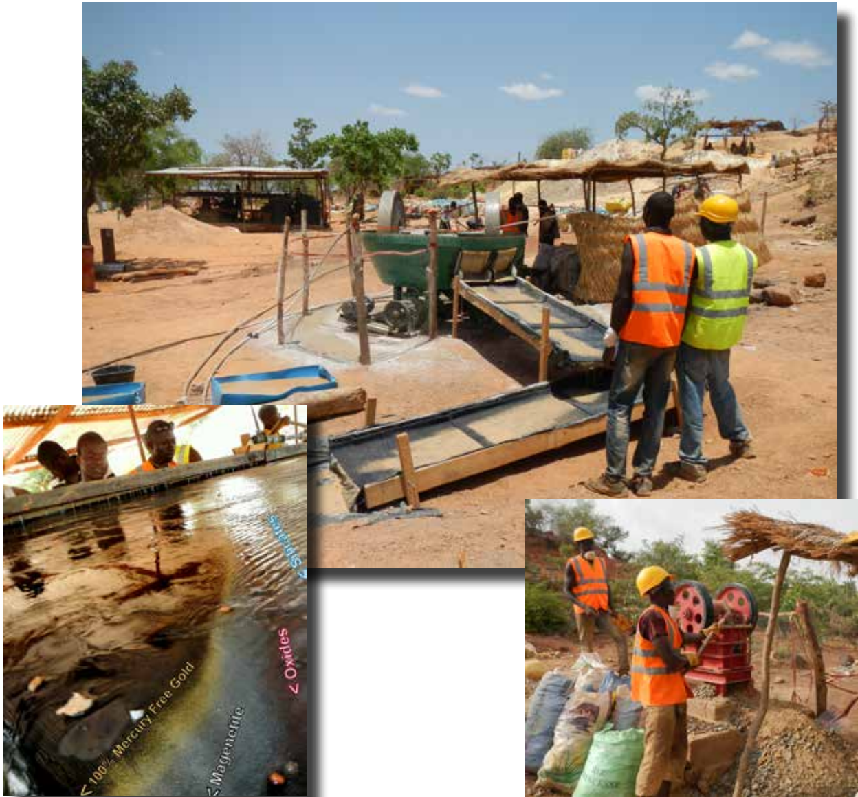
Artisanal Gold Council (AGC) mercury-free artisanal gold production system and training centre in Burkina Faso.
