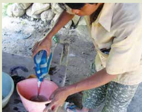
c. Mercury is added to the ore and binds with gold particles to form an amalgam of mercury and gold
