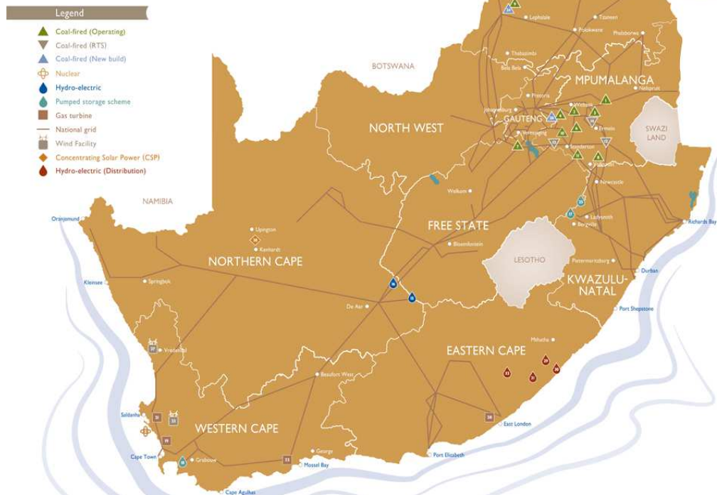
Figure 1. Map showing Eskom power stations in South Africa. Coal-fired stations (green triangles) are concentrated in west-central Mpumalanga Province. Coal-fired stations returned to service (Camden, Grootvlei, Komati) are shown as gray inverted triangles, and future stations (Medupi, Limpopo Province, and Kusile, Mpumalanga Province) are shown as blue triangles. Source: Eskom, www.eskom.co.za .
