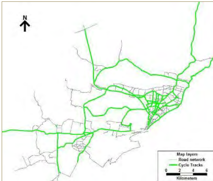
Figure 54 Links with ROW>30m for segregated cycle tracks
