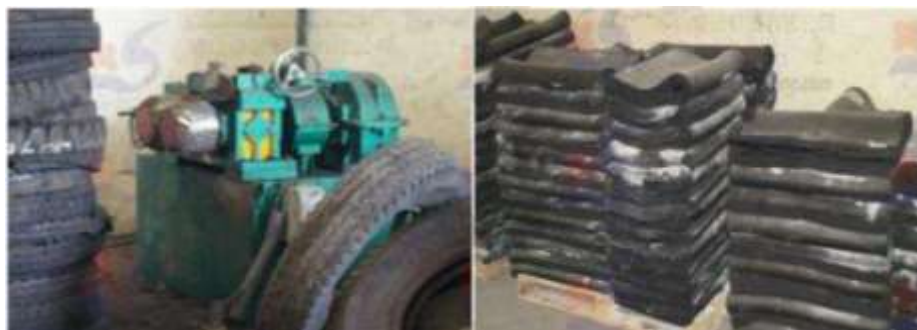
Figure 5.16: Debeader and Cut Rubber for the Footwear Industry, Surabaya, Indonesia 174
