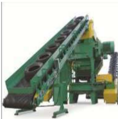
CM Single Speed Tire Shredder – Processes passenger car and SUV tires into a 50 mm clean cut chip at a rate of 8-9 tons per hour.
