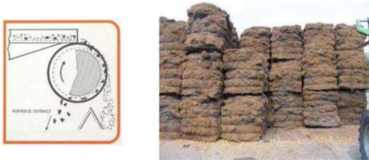
Figure 5.15: Drum Magnet and Metal Separated Magnetically and Baled 166
