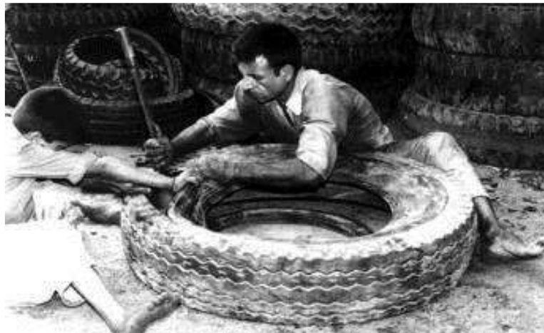
Figure 5.13: Manual Separation of the Tread from the Sidewalls, Karachi, Pakistan © PCSIR – WASTE (left) Manually-loaded tyre debeader manufactured in Jiangsu China, Careddi Technology Co., Ltd.(right)
