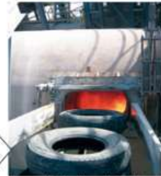
Figure 2] Whole rubber tires introduced directly into the kiln by conveyor as an alternative fuel.
