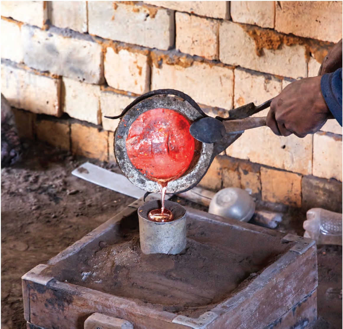
Aluminium is recycled by hand in Ambatolampy, Madagascar. Photo: Dennisvdw © Getty images
