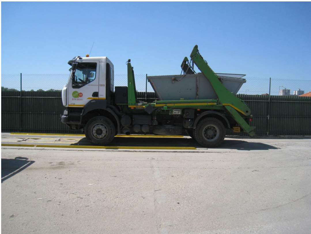
Picture 10: Balancing of container at the acceptance of the waste for disposal
