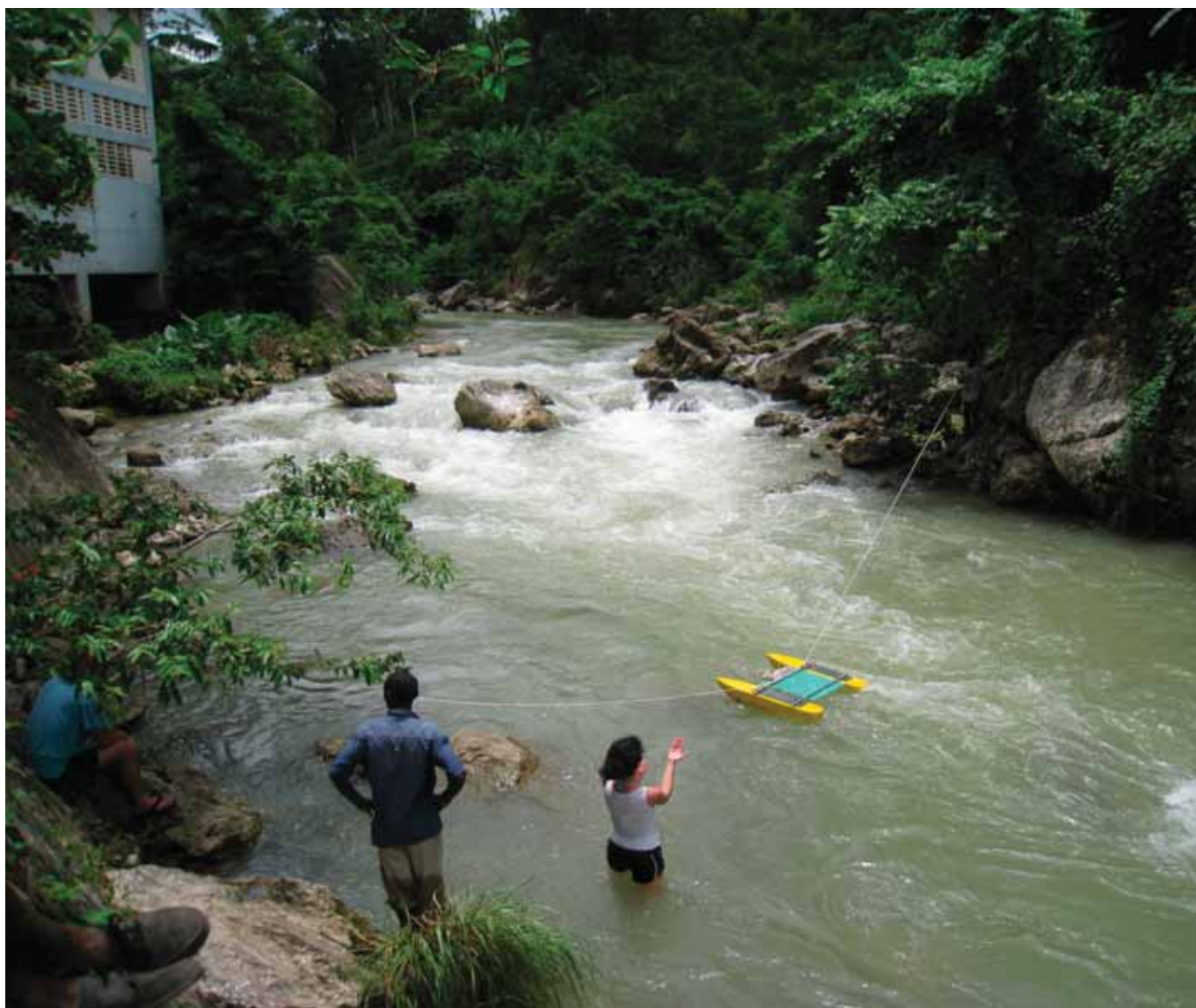
UNEP partners from Columbia University measure river flow velocity in support of a proposed run-of-river hydropower scheme in southern Haiti
