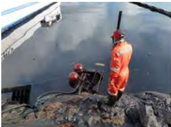
Mechanical oil skimmers operating on oiled shoreline waters, 30 November 2013
