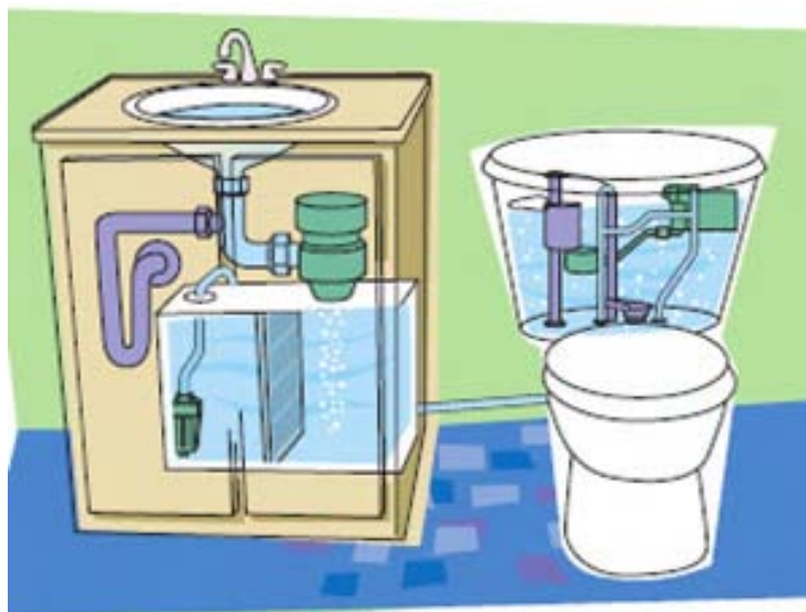
Figure 9: The Aquos™ toilet uses gray water from the sink for toilet flushing.
