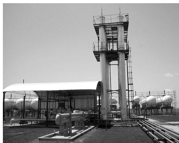
For reference only, this company in Argentina is a supplier of HAPs, they purify LPG and sell HAPs to aerosol fillers. No aerosol filler in the world has columns this big.
