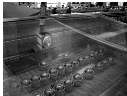
Plexiglas covers protect workers in case a can ruptures.
