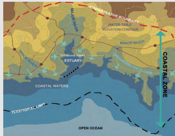
(a) The coastal zone showing the ICZM Protocol boundaries, groundwaters and waters defined by the Water Framework Directive (WFD) (Credit: Brian Shipman, PAP/RAC)
