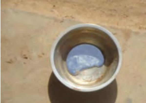
Mercury is used to extract gold from the powdered ore rocks. Photo credit © Awad Siddeg
