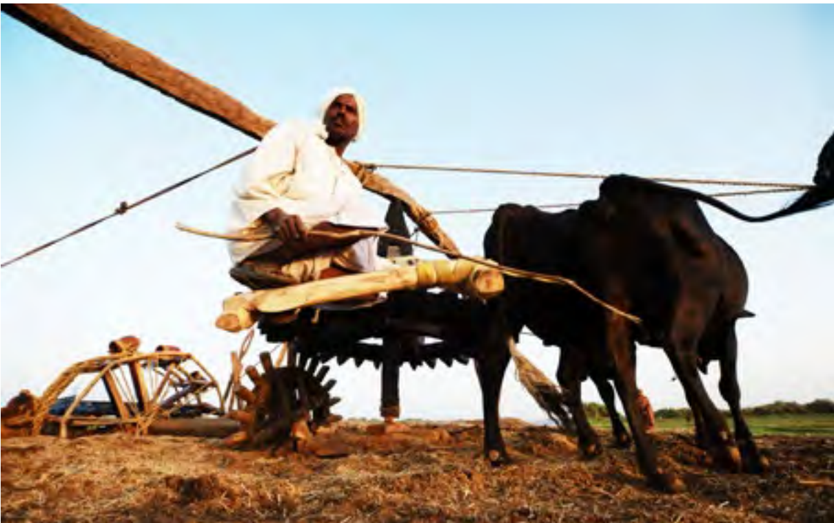
The Saghyia: Traditional water lifting method in Northern Sudan. Photo credit © UNEP
