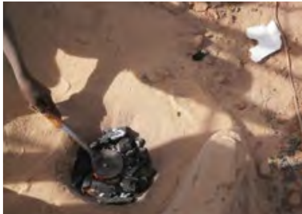
Open heating of the amalgam where mercury sublimes directly to the atmosphere. Photo credit © Awad Siddeg
