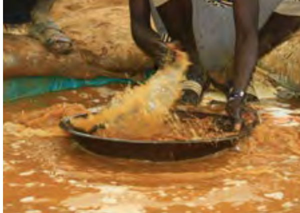
The manual wet processing where mercury and gold combine to form an amalgam. Photo credit © Awad Siddeg
