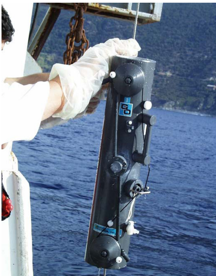
Figure 1 Picture of a GO-FLO sampler (General Oceanics; photo courtesy of IFREMER, France).
