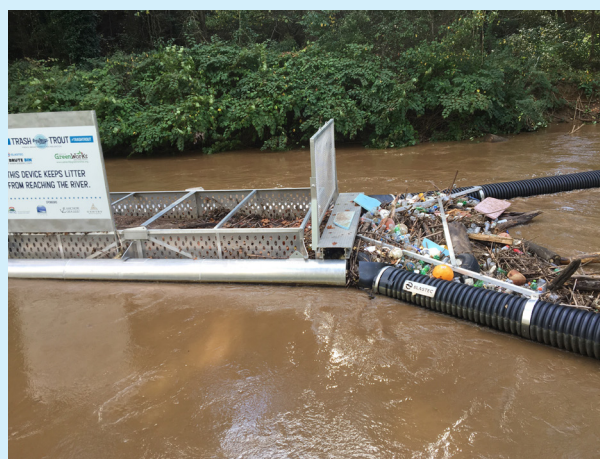
In this example the bin attached to the boom system captures floating trash.
